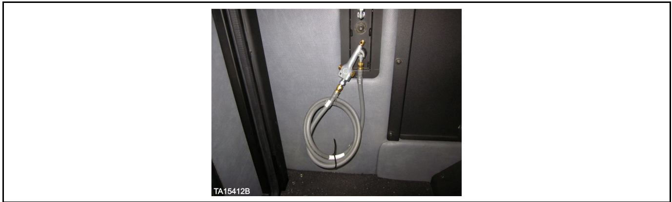
Figure 27: Air cleanout hose location
